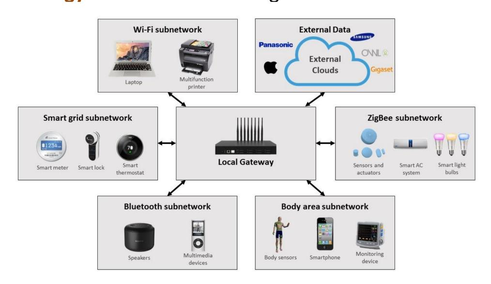
To address the requirements of resource-dependent devices and IoT scenarios, M2M communications require the integration and convergence of different communication systems and protocols.
