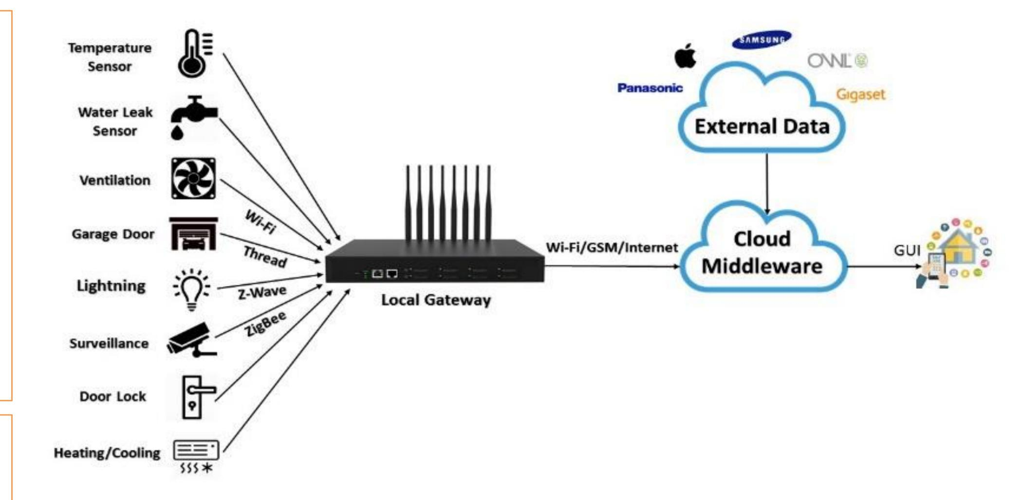
The integration of wireless M2M communications to connect devices located in remote areas even with limited accessibility. A fast and cost effective interconnection between M2M devices can be achieved by using medium-range communication technologies as ZigBee (IEEE 802.15.4), Wi-Fi (IEEE 802.11), Z-Wave and Thread.
