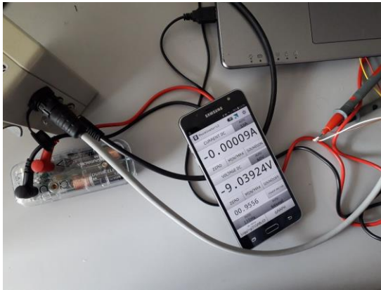
Fig. 9. Parameters generated by A724 when opening the solenoid valve.
