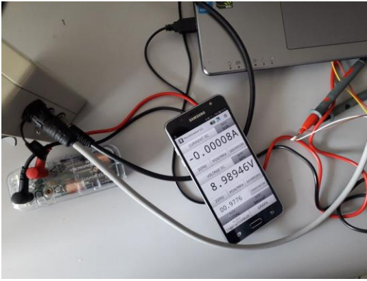
Fig. 8. Parameters generated by A724 when closing the solenoid valve.
